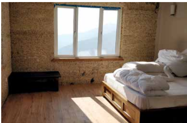
The eco-friendly Yangrima Eco Lodge is built with hemp concrete
